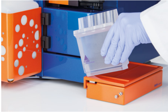
Figure 2.10: Secure the MACS Reagent Rack 4.
