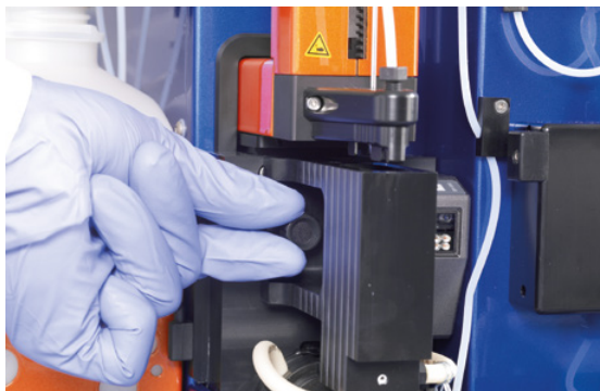
Figure 7.20: Dismantle the washing station.
