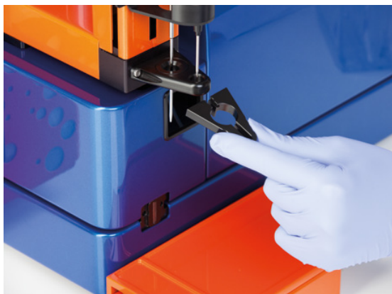
Figure 7.1: Removing the needle guard for cleaning.
