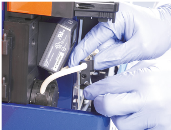
Figure 7.22: Removal of the waste distributor.
