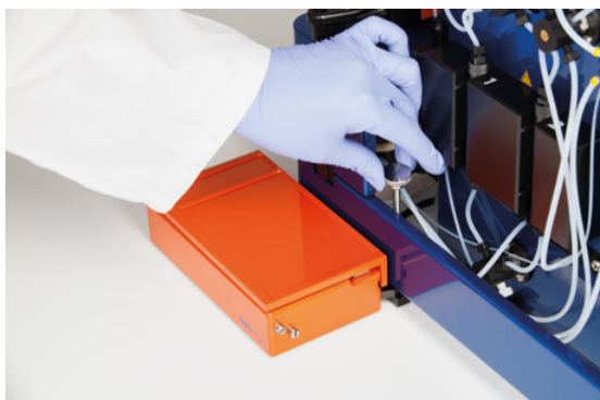
Figure 2.9: Secure the MACS MiniSampler Plus.
